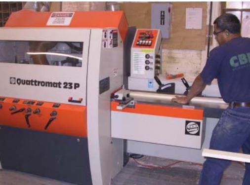
Solid wood parts are processed in the mill room with a Weinig Quattromat 23P moulder, seen here, a Powermatic jointer and Butfering Super widebelt sander.
